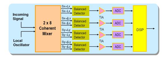
Optoplex's **2x8 Coherent Mixer** is free-space micro-optics-based and patent pending. The device exhibits highly athermal behavior in terms of insertion loss and phase error. When the output signals are detected by four pairs of balanced receivers, both the amplitudes and the relative phase information of the input signal can be extracted for signal amplification and cost-effective compensation of optical transmission impairments, such as dispersion and PMD, in the electronic domain.
